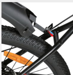
Insert the screws and fender together and tighten
