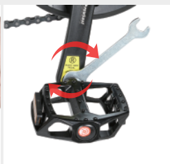
Tighten the right pedal "R" clockwise
