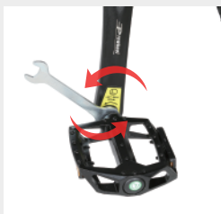
Tighten the left pedal "L" counter clockwise
