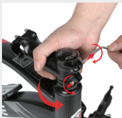
Loosen the two screws and Rotate 180°
