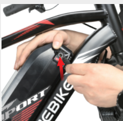
Method 1: Place the battery on the ebike for charging, insert the charging interface into the charging hole according to the direction.
